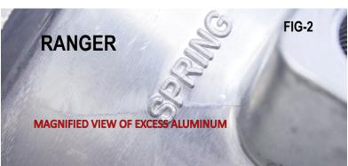
In Fig-3 / 4, you can see that these [markings] are common to all ALUMINUM CENTER ADAPTERS as evidenced by the two OEM-sample photos below...
